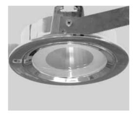
**Body:** The body and frame are aluminum injection designed to enhance the cooling surface. The mounting springs are stainless steel. Body is painted with min. 80 micron powder paint.
