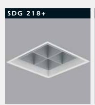
Body: Al quality DKP steel sheet is used, 1 mm thick for front part of the downlight and 0.6 mm thick for back side of the downlight. Painted with 80 micron rainted with 80 micron thick epoxy polyester powder paint. Inner frame is made of aluminium in plus shape to prevent glare.
