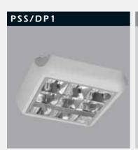
Double Parabolic Bright Louvre: The special form of 0.4 mm thick (99.9%) pure anodized aluminum reflectors offer high efficiency. Double parabolic lamellas produced with the same material are placed in front of the reflectors to minimize glare. Double Parabolic minimize glare.
