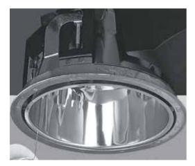
**Body:** Body and gear boxes are manufactured with Poliamid-6 Natural with 30% glass fiber (GFR) additives. The cables connecting the ballast box to the fixture are housed in a spiral pipe. The ballast box is equipped for hanging on the ceiling if needed.
