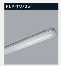
Diffuser: The diffuser is made of UV stabilized, transparent polycarbonate material. It has injection moulded with smooth outer surface and prismatic inner surface. Reflector: The reflector unit has been painted unit has been painted with white polyester and manufactured of 0.6 mm thick DRS steel sheet. It is clipped onto the housing with locking equipment.
