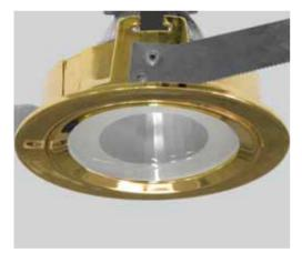
**Body:** The body and frame are aluminum injection designed to enhance the cooling surface. The mounting springs are stainless steel. The body is painted with min. 80 micron powder paint.
