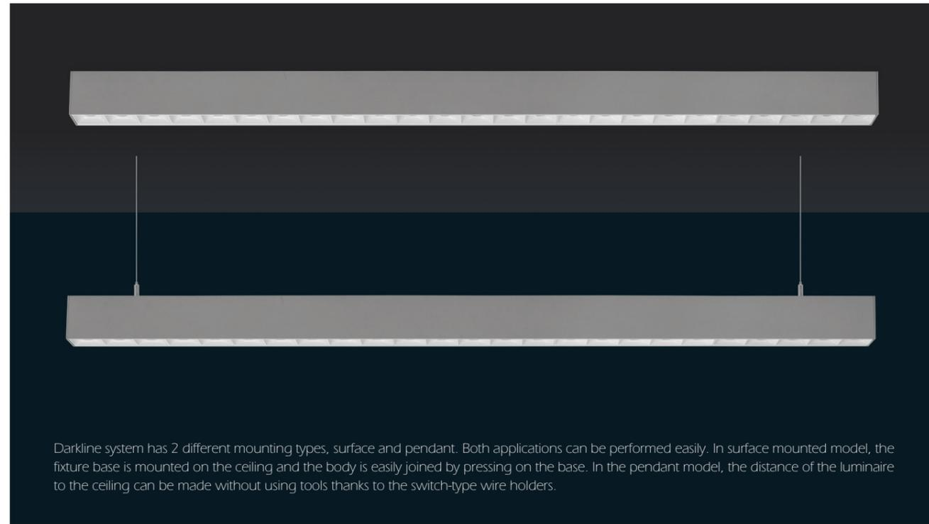
Darkline system has 2 different mounting types, surface and pendant. Both applications can be performed easily. In surface mounted model, the fixture base is mounted on the ceiling and the body is easily joined by pressing on the base. In the pendant model, the distance of the luminaire to the ceiling can be made without using tools thanks to the switch-type wire holders.
